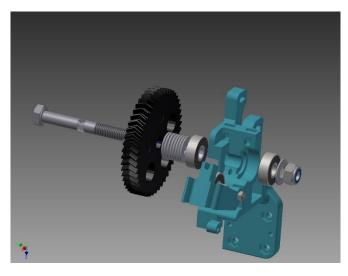
Slide this arrangement though the hole of the extruder body, where another bearing, single washer and M8 nyloc nut need to be placed on the hobbed bolt's end. This order can be seen in the picture.
